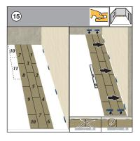
The panels are laid according to the numbering in the image. (Trim the first row if necessary, as described in Figure 10.) In this sequence, the first 3 rows are laid out in the room. This way of laying ensures that the rows are connected in straight lines.
